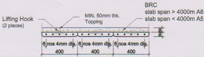
PIC. 3 TYPICAL PRECAST PRESTRESSED SLAB SECTION
