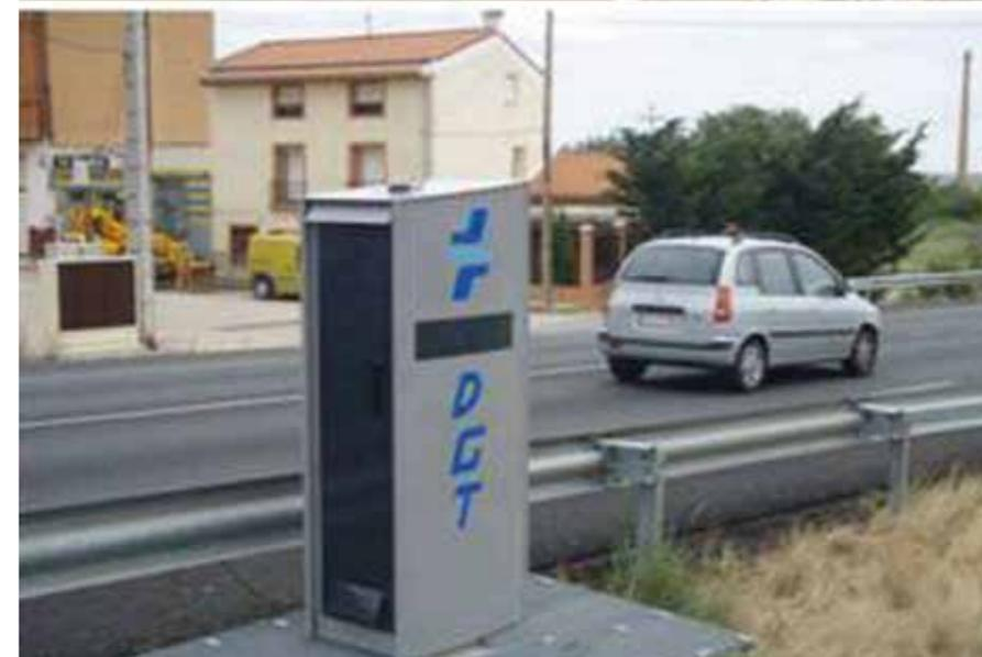
Illustration 1 - ITS devices enforced to control and manage temporary speed limits
