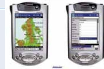
Figure 4 - Hand held data capture tool used to record field data
