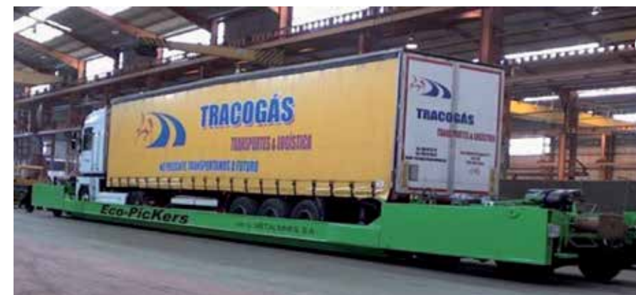
Picture 7 - A system for transferring trailers on to railway called Eco-Pickers developed by MetalSines.
