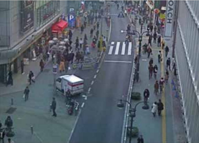
Example in Shibuya-ward, Tokyo, Japan: The width of the road was narrowed and permanent spaces exclusive for loading/unloading were introduced. In addition, regulations were revised in order to oblige buildings with large floor spaces to install loading/ unloading spaces.
