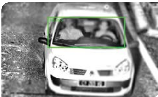
Testing of the sensor to detect the number of occupants in a vehicle crossing the Franco-Swiss border
