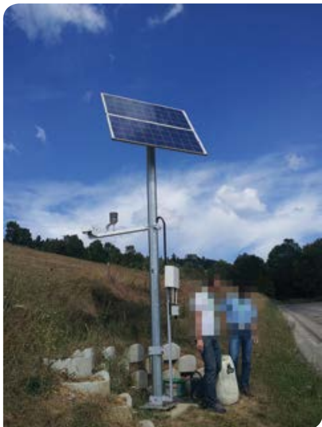
Example of a Roadside Unit - Equipment deployed within the scope of the European project «Syncro» (Isère Department, France)
