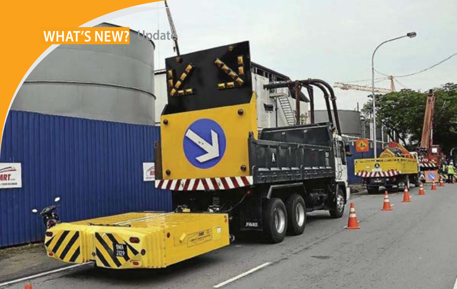
Illustration 5 - Safety measure in road work zone: lorry-mounted attenuator © www.thestar.com
