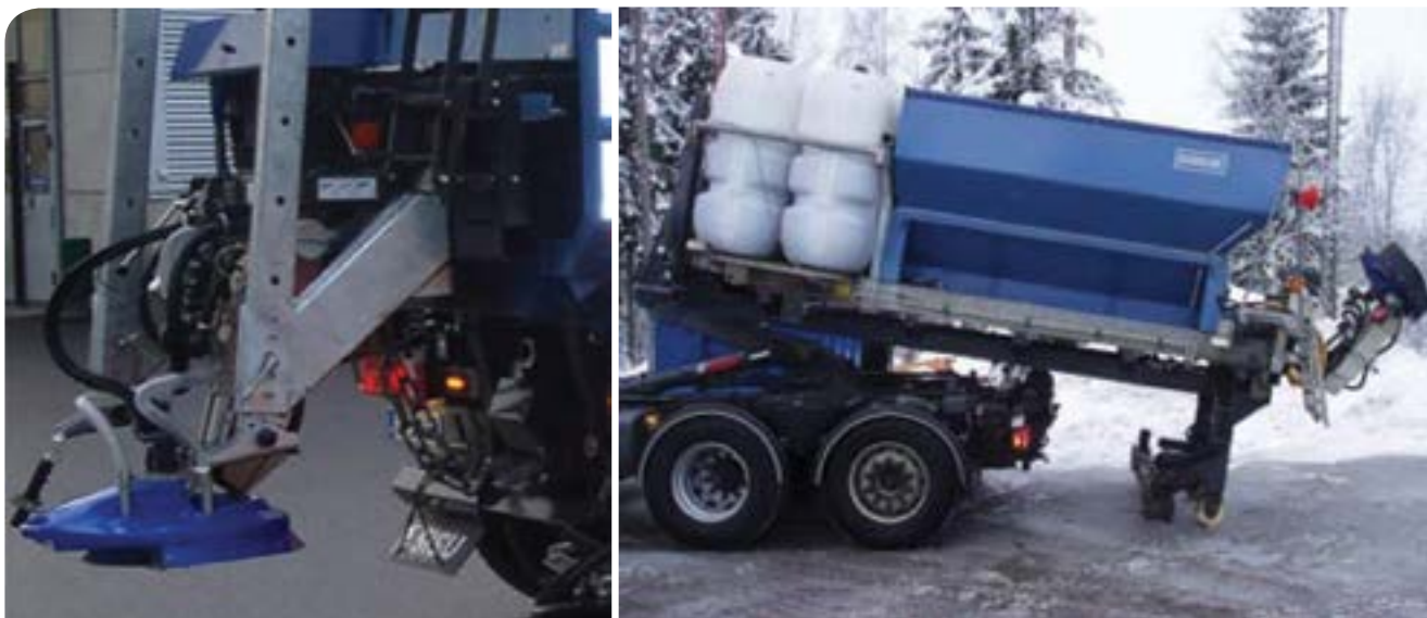
Illustration 6 - Spinner with salt dispenser and separate containers for different materials
