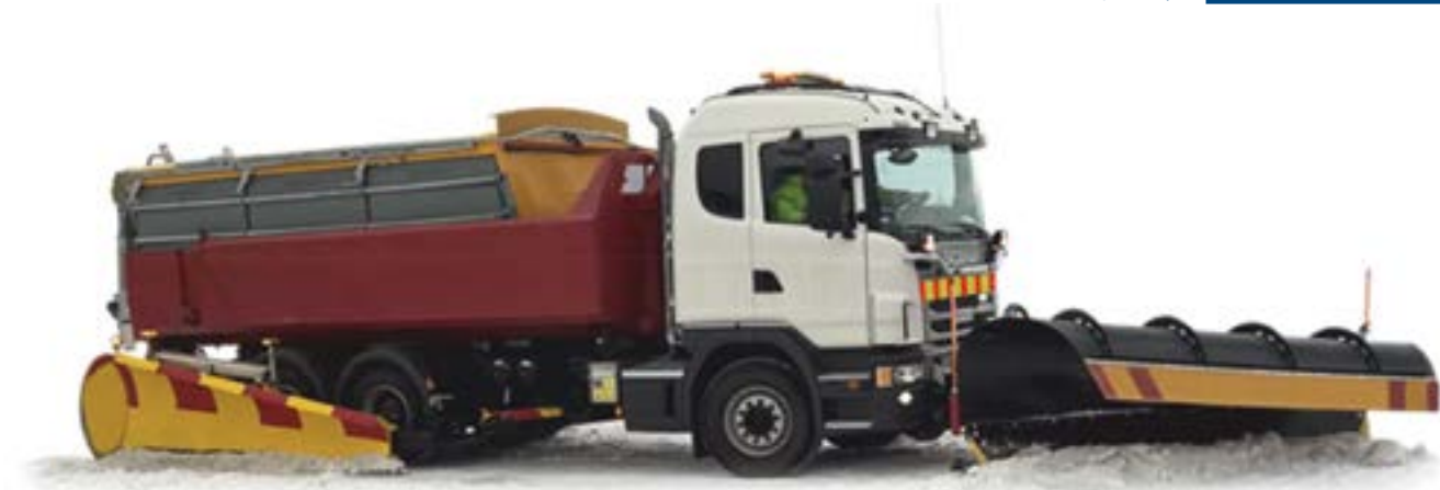
Illustration 5 - Heavy winter maintenance unit, truck with side, underbody and front plough and rear spreader automat
