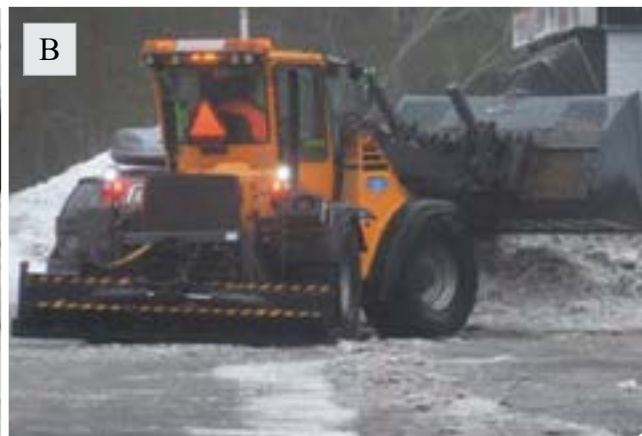
Illustration 3 - Heavy, high-speed truck (A) and small multitask loader for bicycle paths (B)
