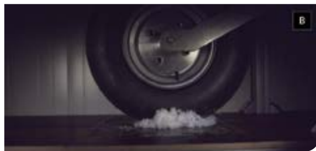
Illustration 2 - Tire Pavement Interaction in water and snow condition
