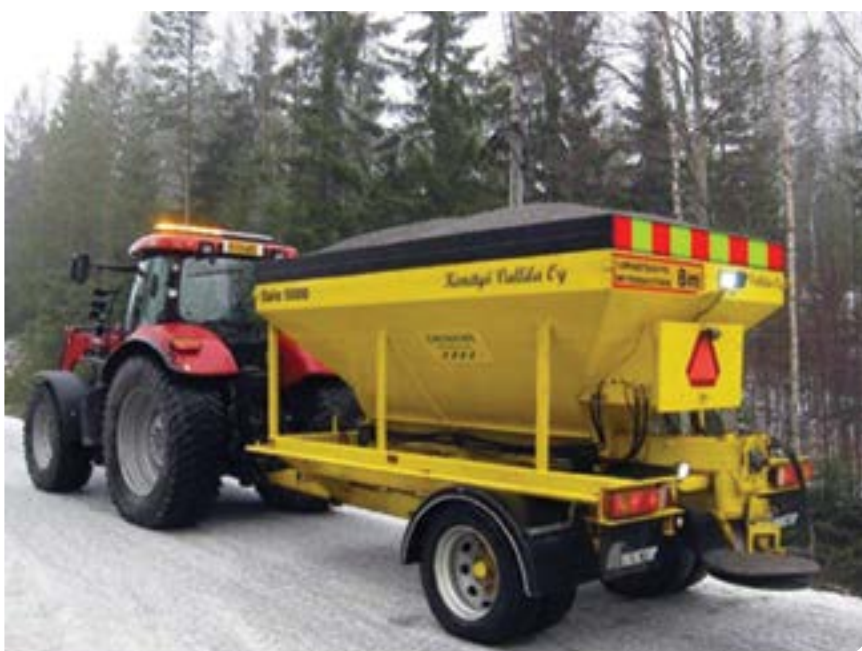
Illustration 7 - V-box with belt feeder for gravel/sand
