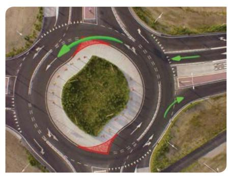
Illustration 1 – Change of direction from a secondary road on turbo roundabouts with a transition to the inside lane © Reddit.com
