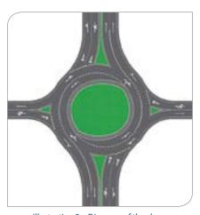
Illustration 2 – Diagram of the channelized spiral roundabout or turbo roundabout with a transition to the inside lane
