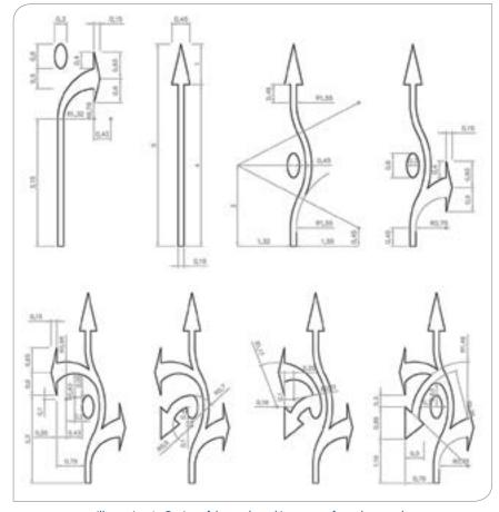
Illustration 4 – Design of the road-marking arrows for turbo roundabouts with a transition to the inside lane
