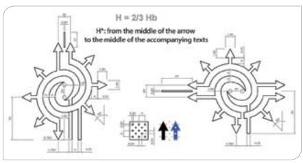
Illustration 3 – Design layout of signs for turbo roundabouts with a transition to the inside lane
