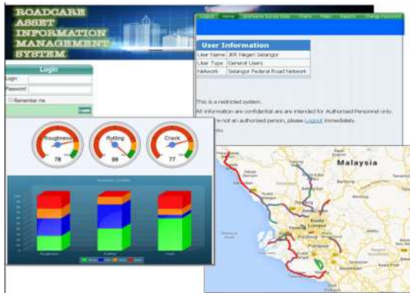
Figure 4.2 An example of visualisation of a condition score of pavements in a network, using a set of PIs (roughness, rutting, cracks); the interview with Roadcare, Malaysia.
