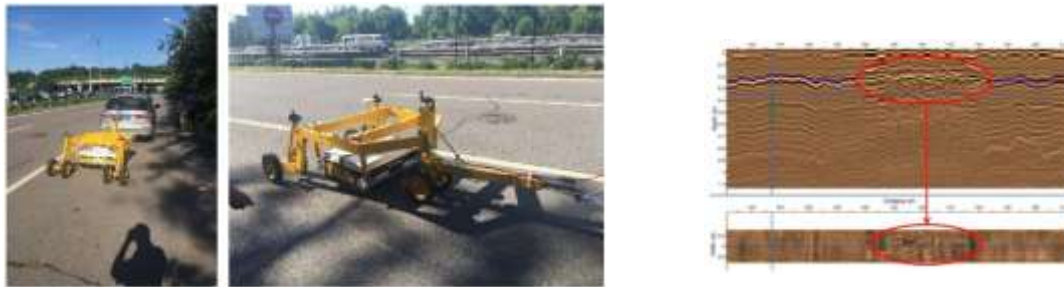
Figure 4.12 3D-Radar during inspection (left), and an example of radar image showing reflective cracking (right); JSTI Group, China.
