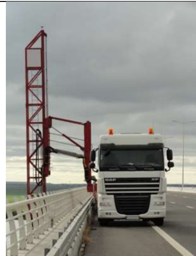
Lighting provided in central reserve which permits use of under bridge inspection vehicle.
