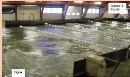
3D model representing wave surges (dike on the left, wave-making machine on the right) - ©Egis
