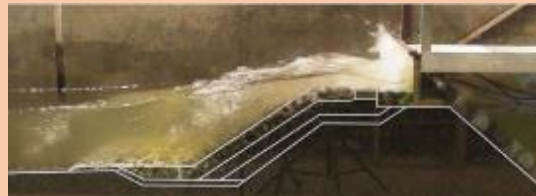
Efficiency of the sea wall for waves protection using a 3D model - ©Egis
