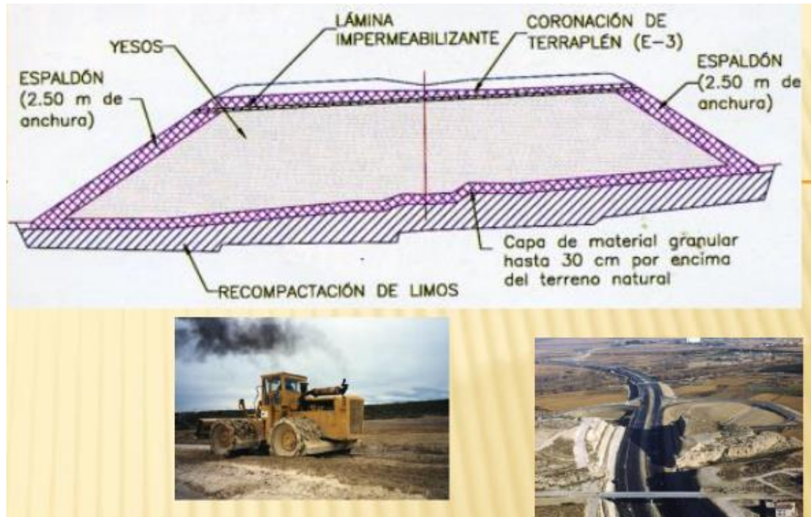
Figure 7.1: Highway A23 Villanueva de Gallego-Zuera (Spain) – Embankments geometry and materials.
