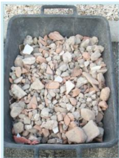
Figure 5.3: Materials coming from C&D waste; 1 – Coarse for structural use, 2 – Coarse for filling, 3 – Mix for structural use, 4 - Sand
