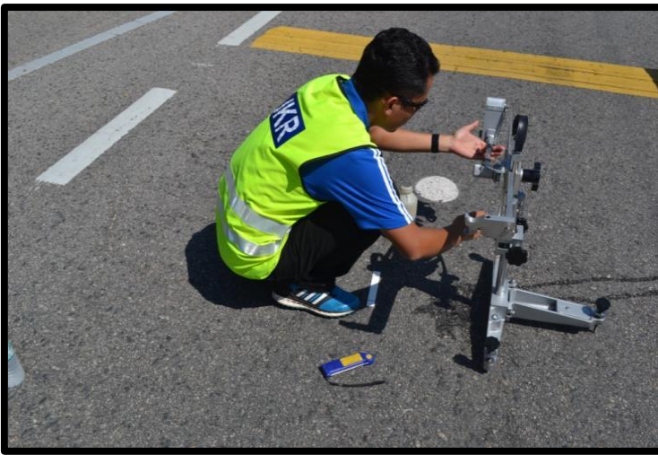
Picture 2: Skid Resistance Values Are Measured using British Pendulum Skid Tester. The test is conducted based on ASTM E303-87.
