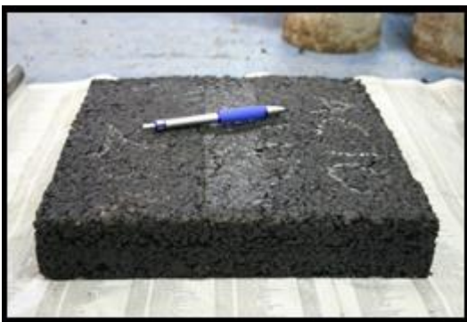
Asphalt performance test using PMA has a better resistance to rutting
