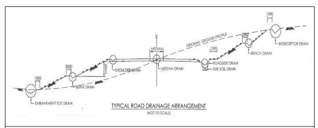
This is the typical road drainage arrangement for cut and fill embankment. Consideration should be given to the possibility of water flowing towards the roadway, either on the surface or through the water bearing strata. Care should be taken to keep ground water table below the formation surface and prevent erosion or slope failure.
